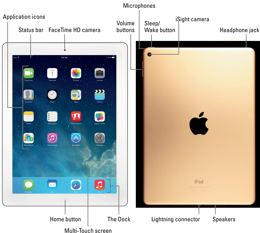
Figure 2-2: There are probably fewer gizmos to get used to on an iPad than on the average cellphone.
