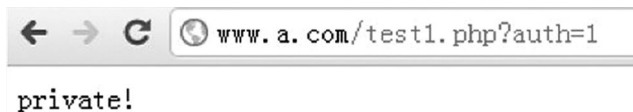
FIGURE 14.14 Change the value of the variable $auth and bypass the logic on the server side.
