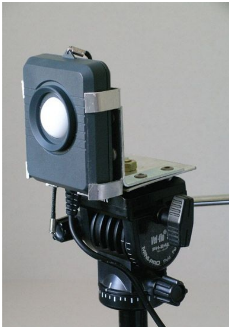
Figure 6.13 A photometer head mounted on a right-angle bracket, onto a photographic tripod.
