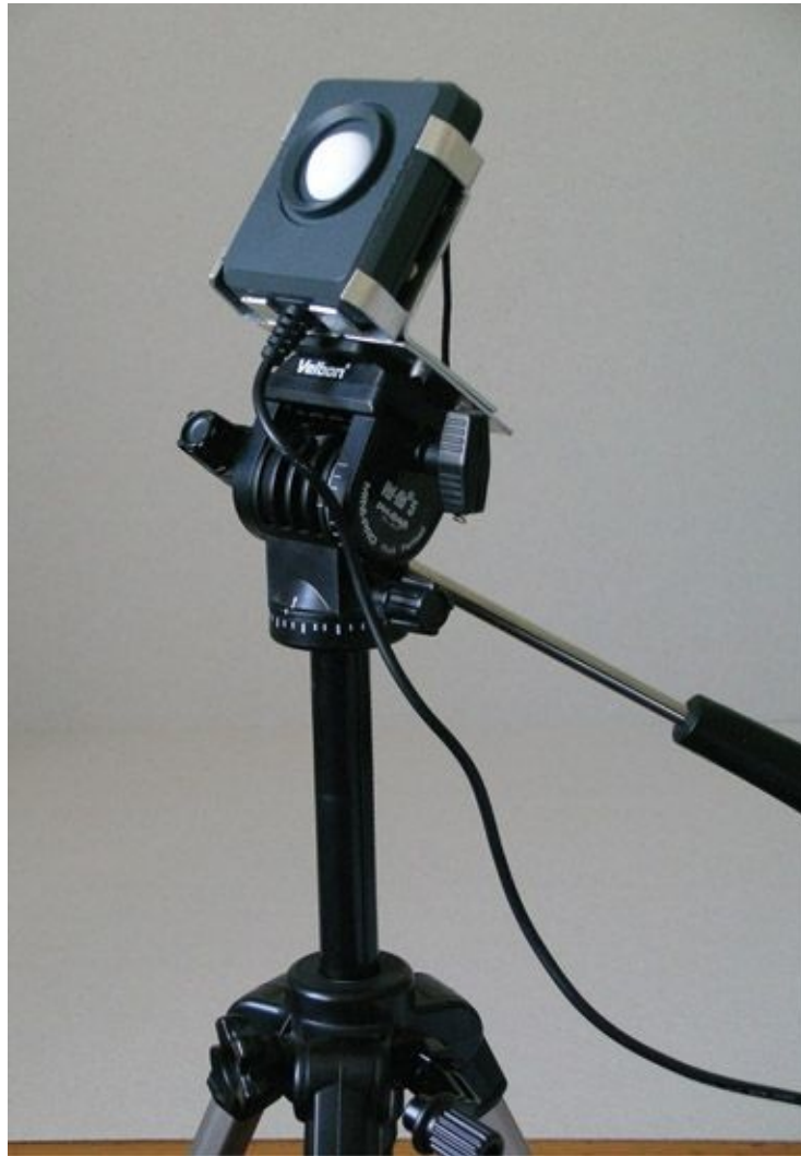
Figure 6.14 The photocell tilted to +35° relative to the horizontal plane, and ready for measuring the three-dimensional illumination distribution.
