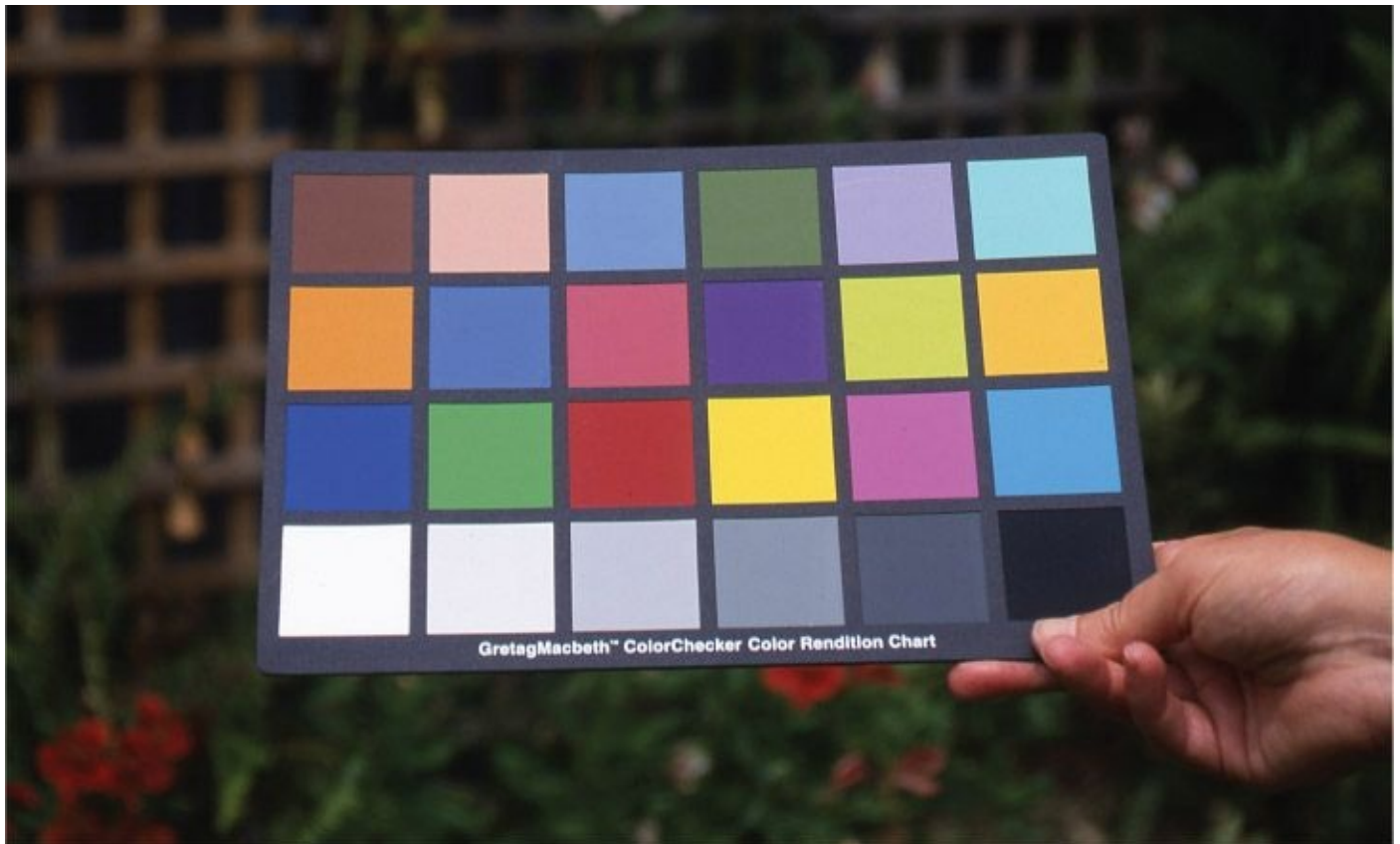
Figure 4.12 The GretagMacbeth ColorChecker colour rendition chart being examined under daylight. A viewer who forms a clear memory image of the chart in this situation can then make comparisons with its appearance under other sources of illumination.
