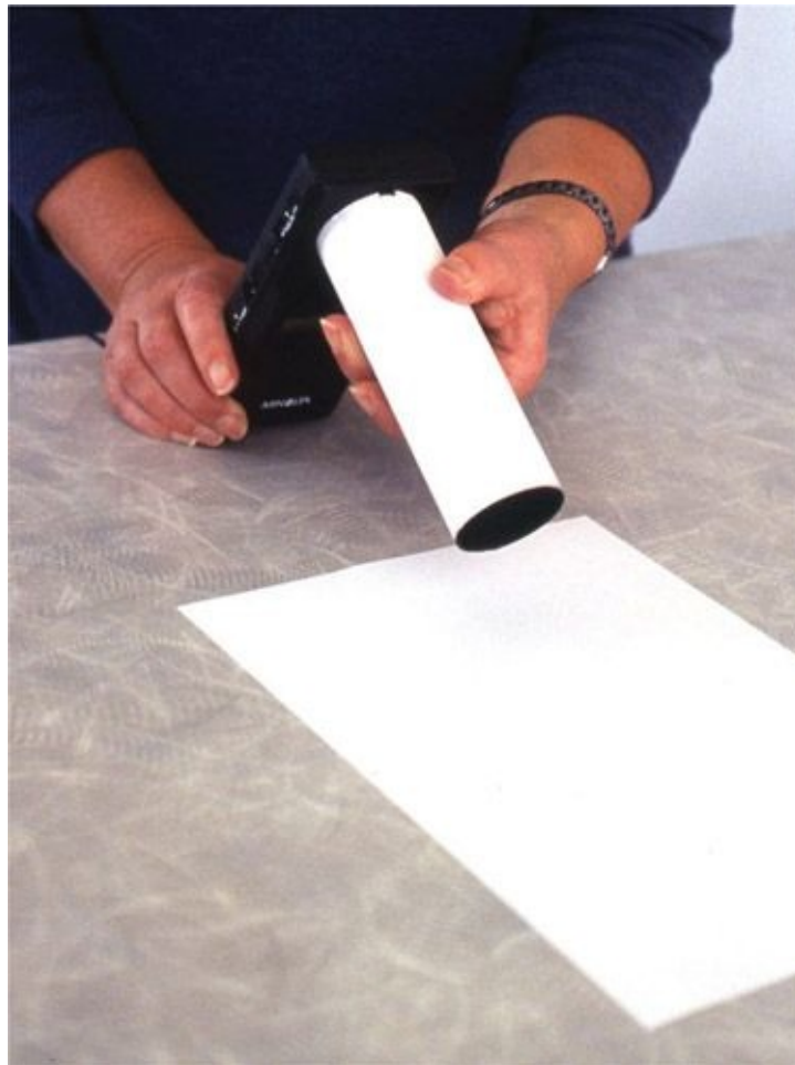
Figure 2.8 Using an internally blackened tube mounted onto a light meter to obtain a measurement of surface reflectance. Two measurements are made without moving the meter, one of the surface as shown, and a comparison reading with a sheet of white paper in the measurement zone.
