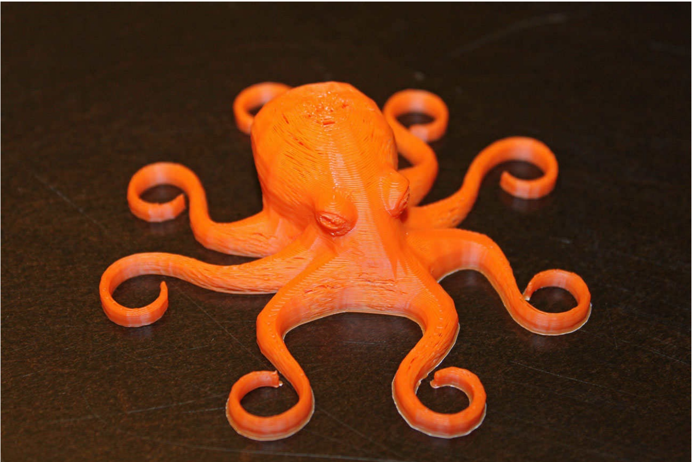
Underextrusion makes the filament strands too thin, causing gaps, as you can see in this printout of an octopus.
