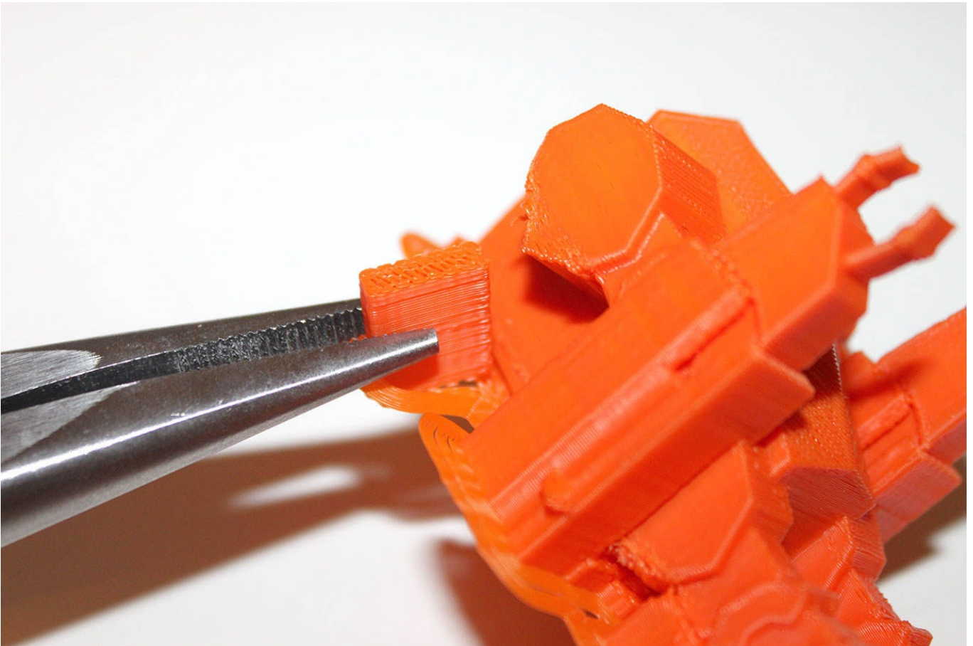
A pair of pliers can help you remove the supports from the model.
