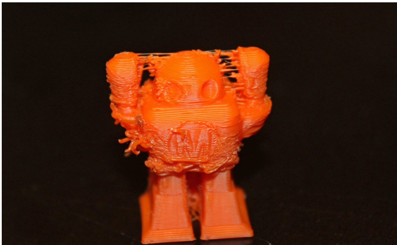
Turning on retraction will usually fix stringing problems like what's shown on this robot.
