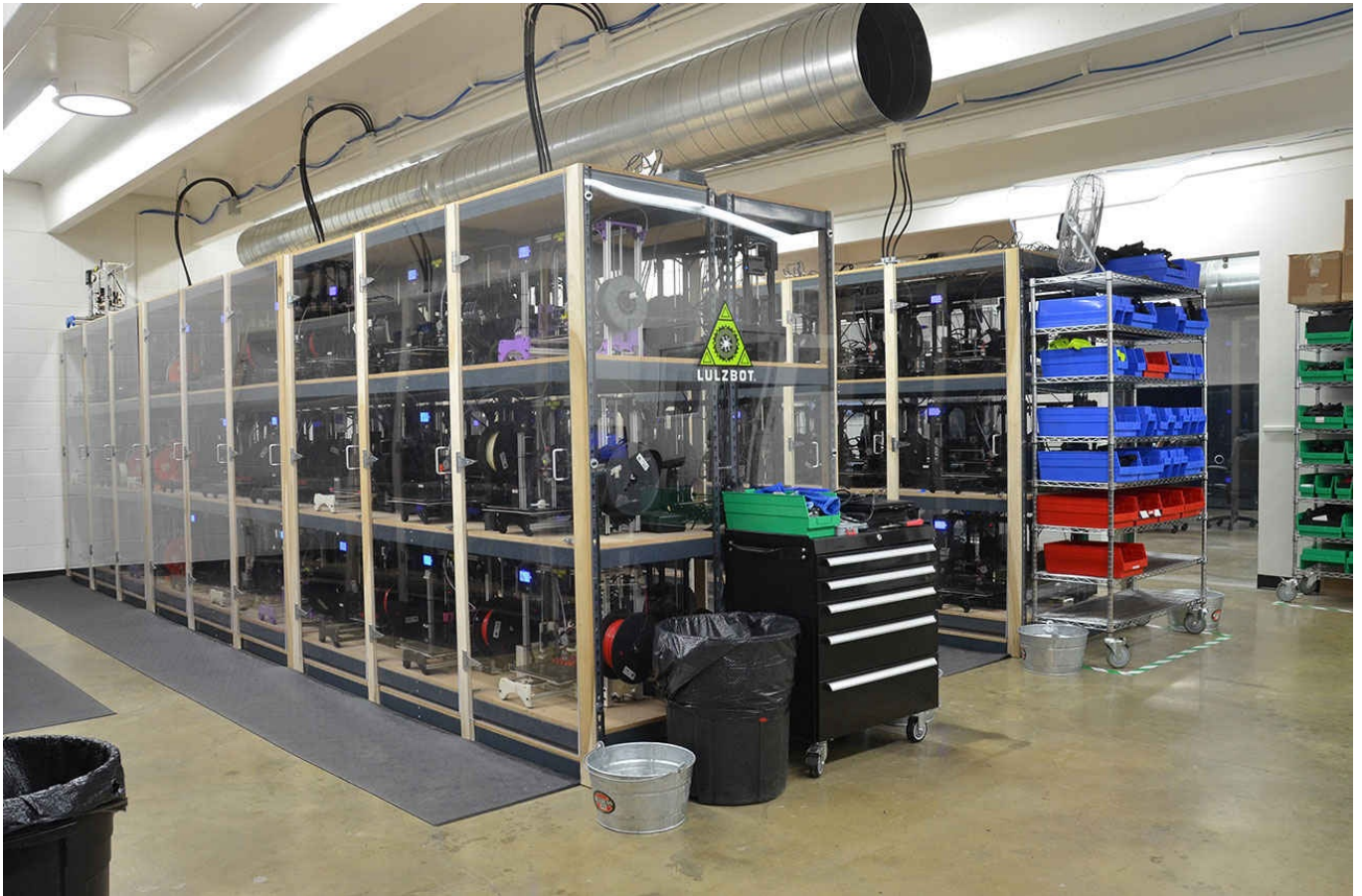
The cluster of 135 3D printers used for manufacturing at Aleph Objects. (Photo courtesy of Aleph Objects)
