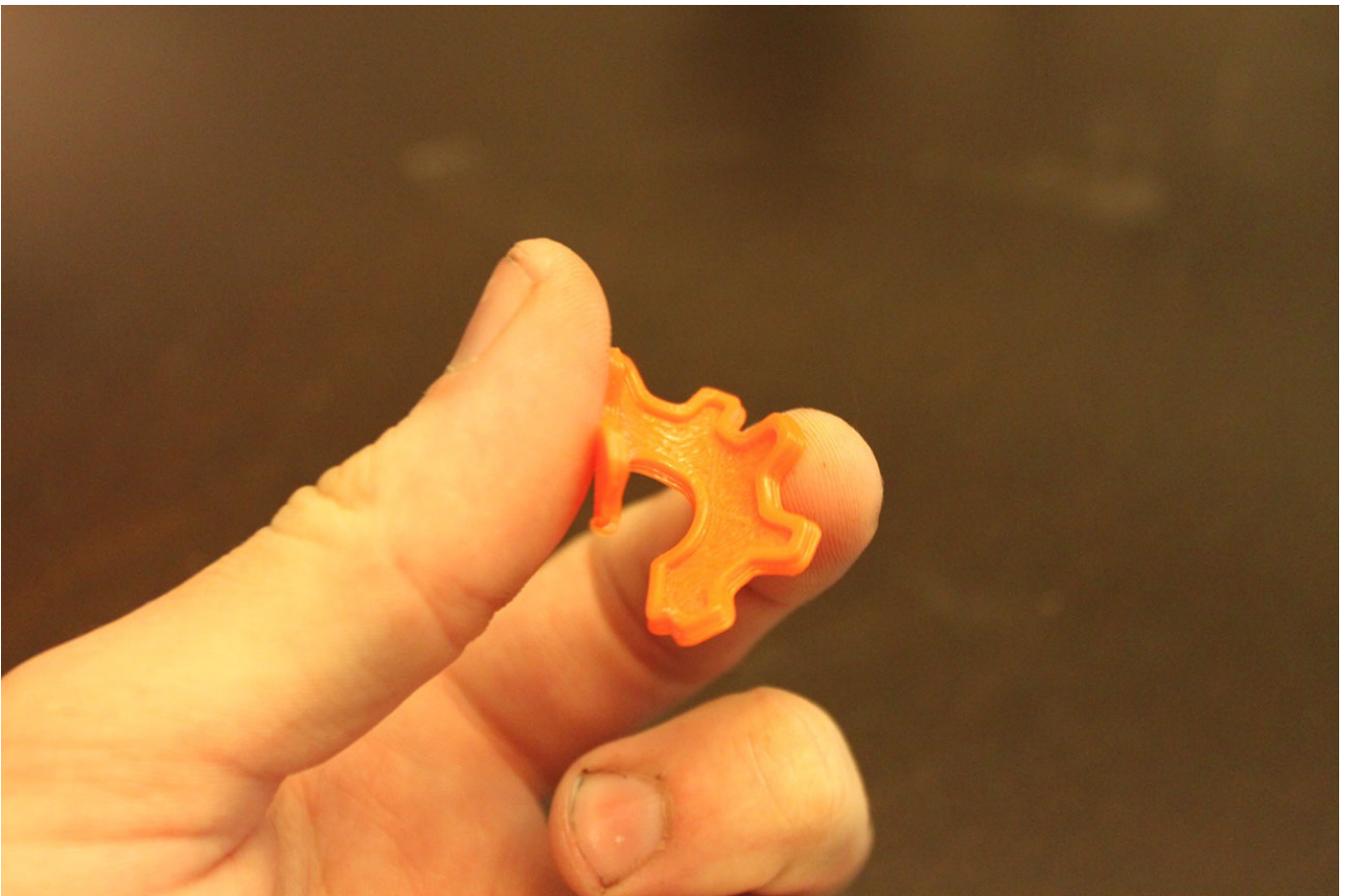
This part was made from NinjaFlex, a popular brand of flexible filament.
