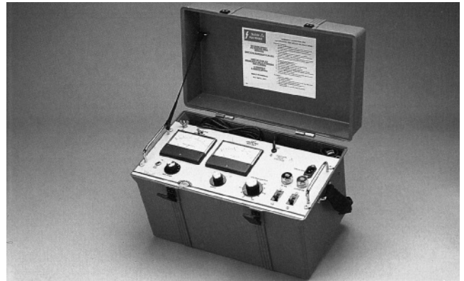
FIGURE 11-28 A dielectric test set.
