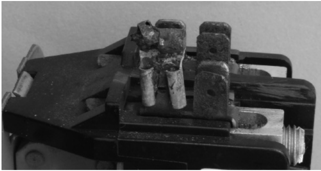
FIGURE 4-4 Overheating caused by a poor connection.
