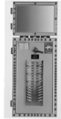
FIGURE 19-12 Explosionproof circuit-breaker panelboard: used in Class I, Groups C, D; Class II, Groups E, F, G; and Class III.
