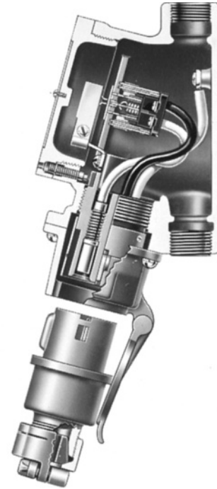
FIGURE 19-25 Cutaway view of explosionproof receptacle.
