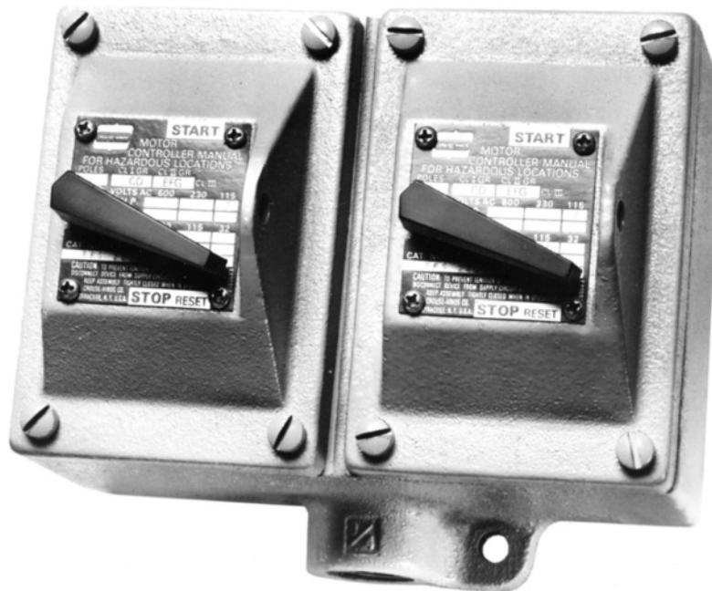
FIGURE 19-19 Dual manual motor starter used in hazardous locations: used in Class I, Groups C, D; Class II, Groups E, F, G; and Class III.
