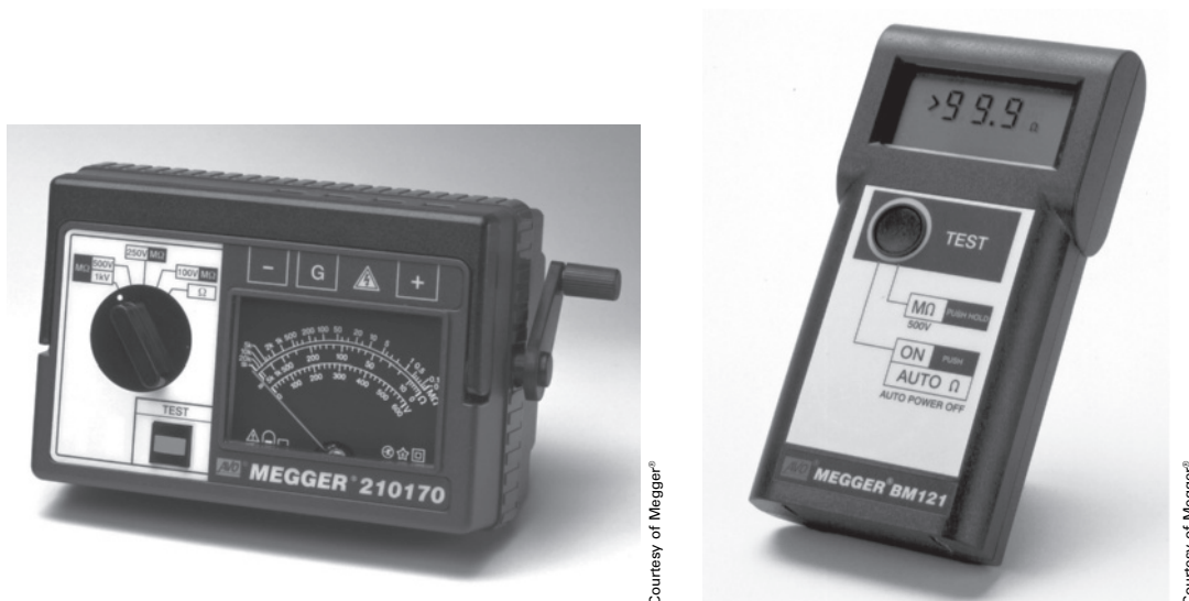
FIGURE 2-42 Meggers used to test transformer windings.
