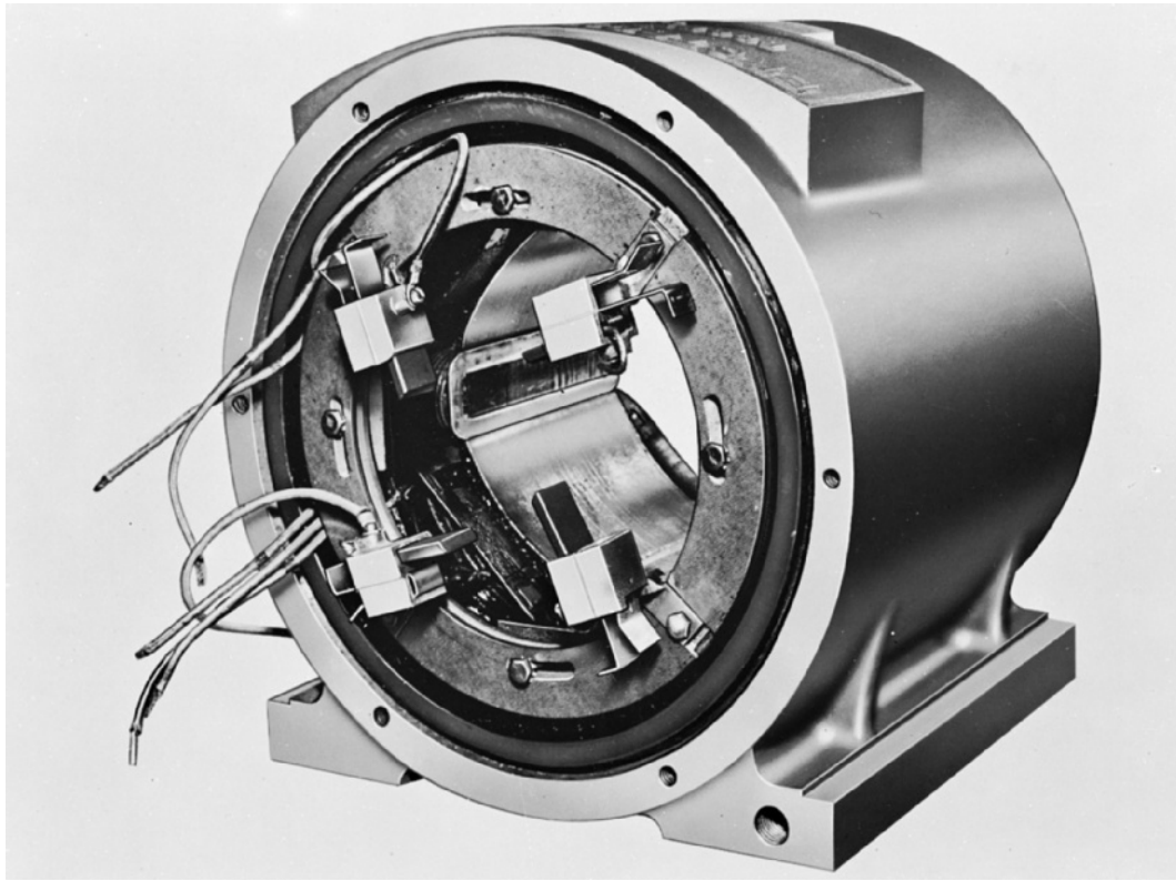
FIGURE 9-42 Field frame of a DC motor.
