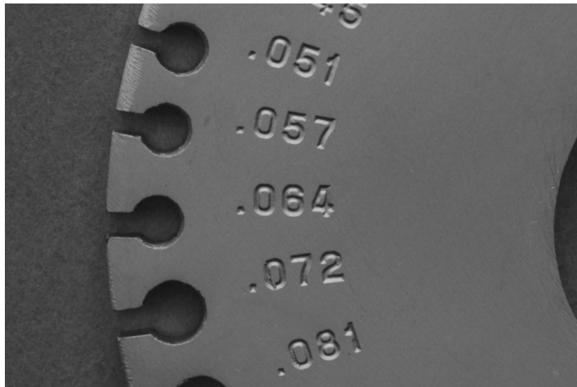
FIGURE 6-15 The opposite side of the wire gauge lists the diameter of the wire in thousandths of an inch.
