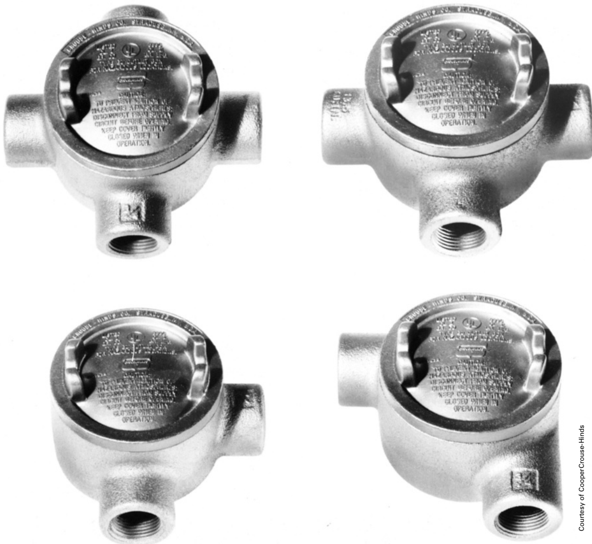
FIGURE 19-3 Explosionproof outlet boxes: used in Class I, Groups C, D; Class II, Groups E, F, G; and Class III.
