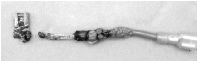
FIGURE 4-5 Burned conductor and terminal caused by a poor connection.
