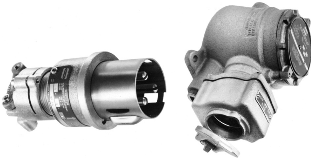
FIGURE 19-26 Explosionproof attachment plug and receptacle: used in Class I, Groups B, C, D; Class II, Groups F, G; and Class III.
