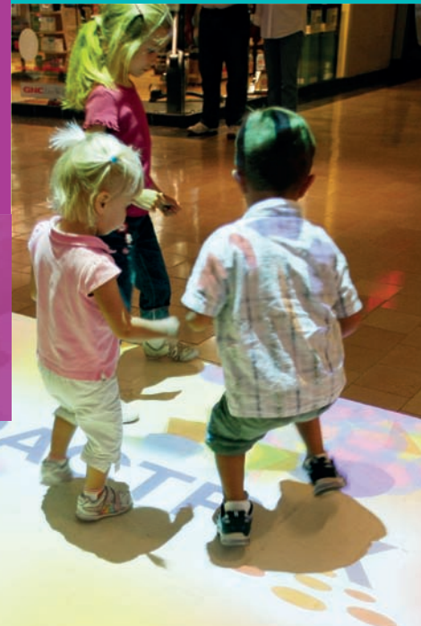
→ Step on it Children play on a Reactrix StepScape interactive ad. As it senses movement, the ad changes its display to produce a simple game or activity.
